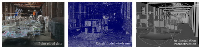
Figure-2 From point cloud to High-precision model
