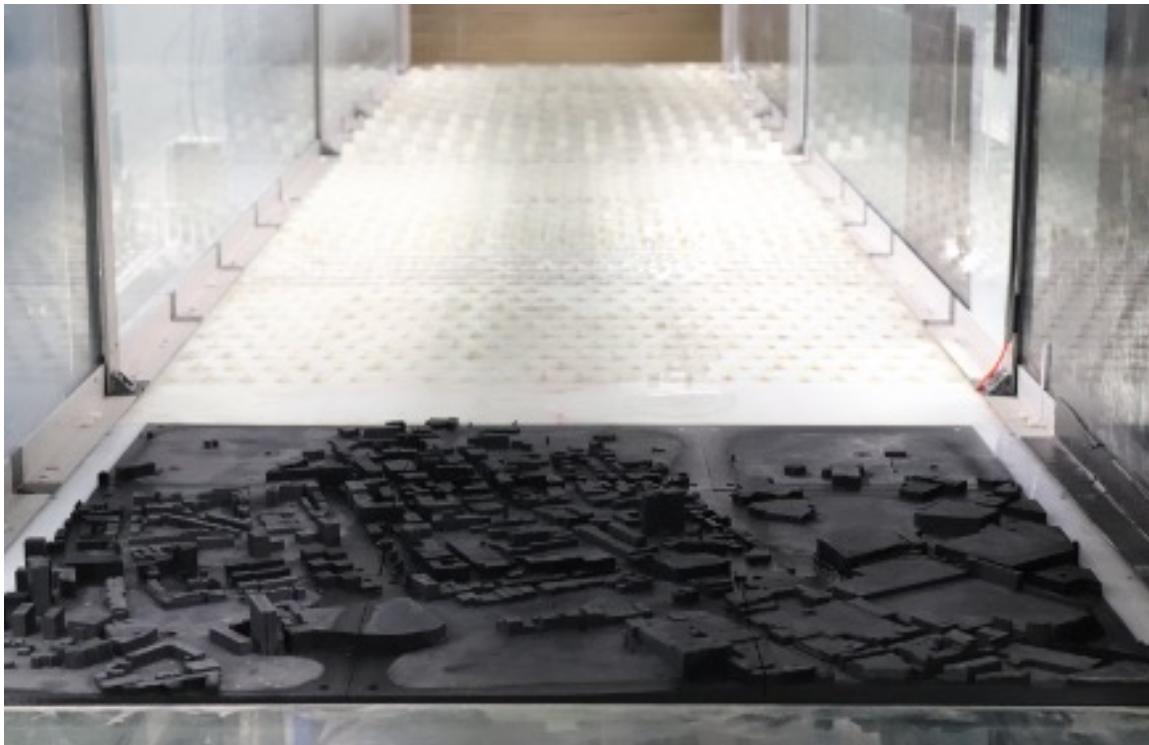
FIGURE 6.2: An image of the experimental setup. In this image, the upstream roughness elements are visible, followed by the 3D printed city model.
