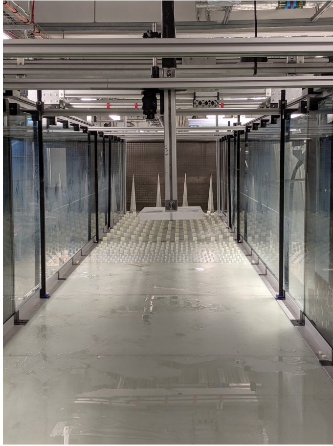
FIGURE 5.4: A photo taken inside the University of Southampton's recirculating water tunnel while fully drained. This photo is taken from the test section looking upstream, it shows the upstream roughness and spires used to generate an incoming atmospheric boundary layer.
