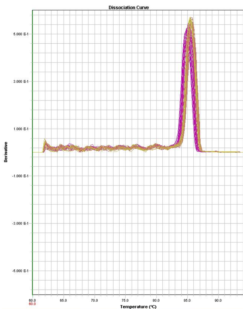
Figure 2.3 Example primer dissociation curve. Presenting a primer pair that produces no primer dimers.
