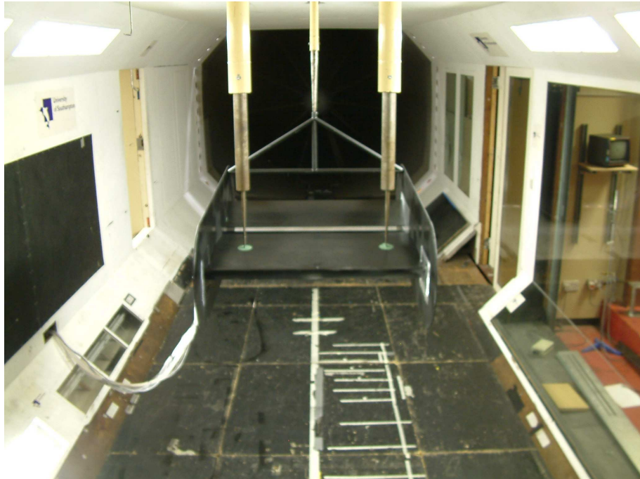
Figure 2.8: Model mounted in the R. J. Mitchell wind tunnel.
