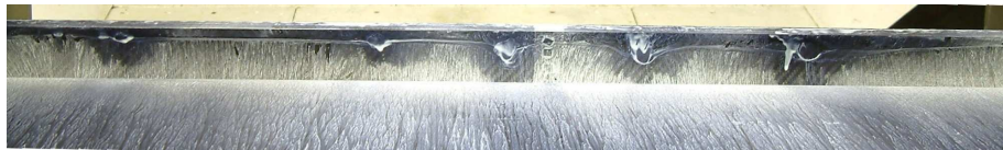
Figure 4.4: Oil flow photograph of the separation line in the cove in the reference conditions. Flow towards the camera, free transition.
