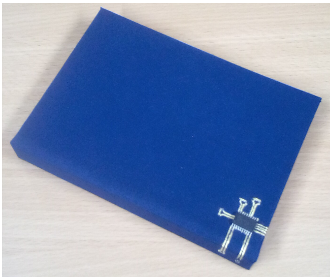
Fig. 6. The complete, case bound book, featuring a microcontroller, four LEDs and a button mounted to the cover, with connections routed over the hinge between front cover and spine.
