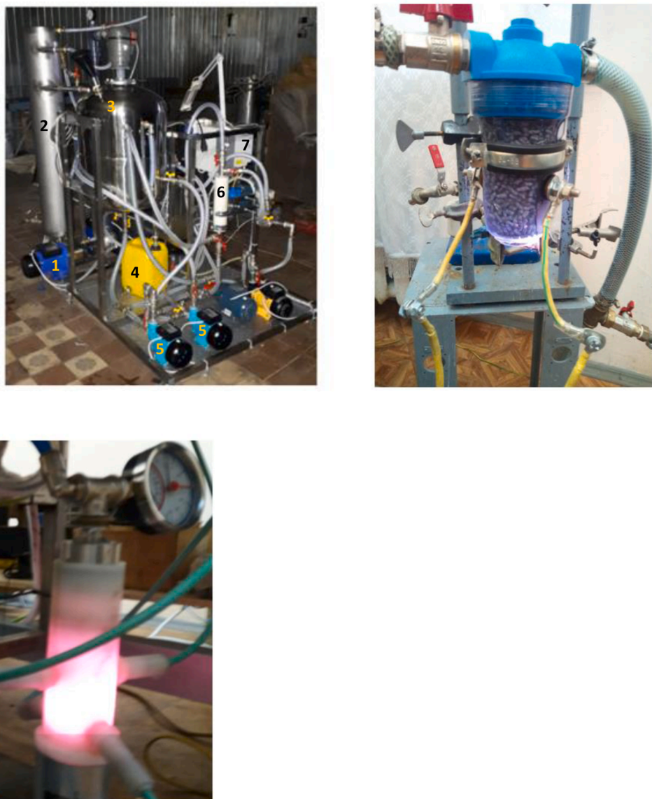
Fig. 3. Upper panel: Left: General view of the assembled treatment system. Key components are numbered as follows: 1 – water pump; 2 – plasma treatment unit (with plasma reactor inside); 3 – filtration unit; 4 – container with concentrated LRW; 5 – microbubble aerators; 6 – outlet filtration unit; 7 –electronic plasma control unit. Right: detail of the non-thermal plasma flow-through reactor (transparent walls show the iron granules loaded into the reactor). Lower panel image shows the plasma reactor in operation. The internal diameter of the plasma unit is 40mm.
