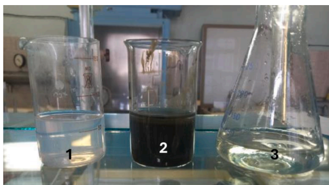
Fig. 4. Liquid radioactive waste samples: 1 – before plasma treatment; 2 – after plasma treatment with suspended iron-rich particles; 3 – purified treated water (after final filtration).
