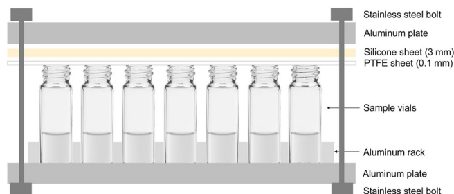
FIGURE 2 Experimental setup for sealing reaction vials during the oxidative conversion of organic nitrogen to nitrate. To seal vials during conversion, up to 120 vials are placed in an aluminum rack and covered with a 0.1 mm–thick Teflon sheet followed by a silicon mat. This stack is squeezed between two aluminum plates by means of threaded bolts to provide a good seal on all vials simultaneously. This setup substitutes the previously used phenolic caps that were manually lined with 0.1 mm polytetrafluoroethylene septa. By making use of easily accessible materials, it represents a cost-effective setup that reduces consumables costs and increases sample throughput. [Color figure can be viewed at wileyonlinelibrary.com ]
