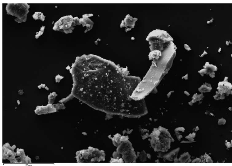
Fig. 7. Scanning electron microscopy image (Hitachi SEM) of sample SV_01 showing that the thoracic fraction (<10 \mu\text{m} ) ash particles are mostly blocky and angular in shape, with smaller particles adhering to larger ones. Scale bar is 25 \mu\text{m} .
