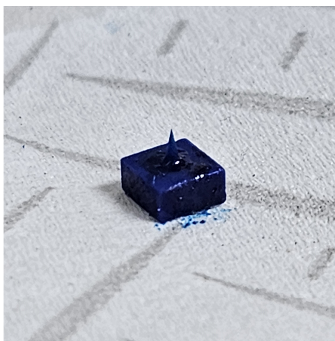
FIGURE 5.36: Emitter 16 after the filling process.
