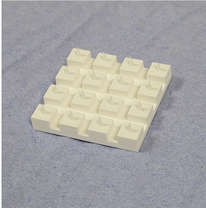
FIGURE 4.7: A block of 16 emitters after CNC manufacturing. The bottom of this block was removed using sandpaper to separate the emitters hence produce 16 individual emitters in a cost-effective manner.
