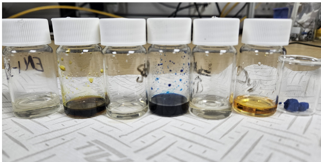
FIGURE 5.1: Appearance of the different ionic liquids, from left to right; EMI- \text{BF}_4 , EMI- \text{FeCl}_4 , EMI- \text{SbF}_6 , (\text{EMI})_2\text{-Co}(\text{SCN})_4 , \text{C}_6(\text{mim})_2\text{-(Im)}_2 , (\text{C}_6\text{mim})_3\text{-Dy}(\text{SCN})_6 and \text{C}_6(\text{mim})_2\text{-Co}(\text{SCN})_4 .
