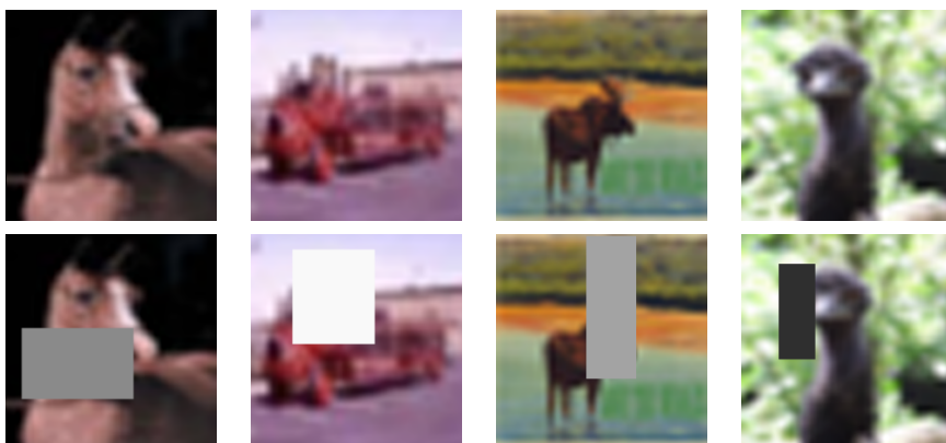
FIGURE 2.11: Data augmentation by the random erasing technique. The first and second rows represent the given images (from CIFAR-10) and the images after random erasing, respectively.
