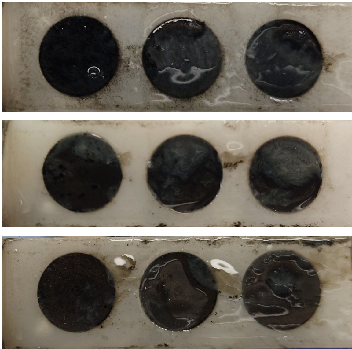
Figure C3b. Photographs taken of the coupon rods taken from the biotic condition on Day 28, on dismantling the reactor, after exposure to anaerobic MB media for 28 days.
