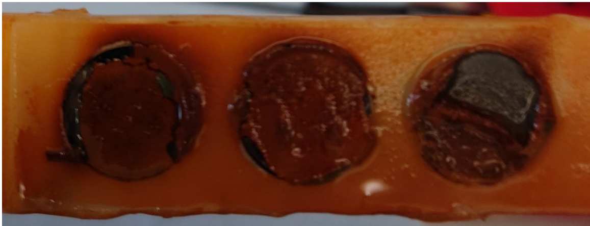
Figure B3a. Photographs taken of the coupon rods taken from the abiotic condition on Day 28, on dismantling the reactor, after exposure to anaerobic nutrient-enriched artificial seawater media for 28 days.
