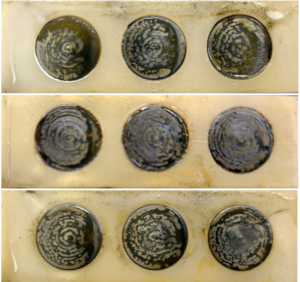
Figure D2b. Photographs taken of the coupon rods taken from the biotic condition on Day 28, on dismantling the reactor, after exposure to anaerobic produced water media for 28 days.
