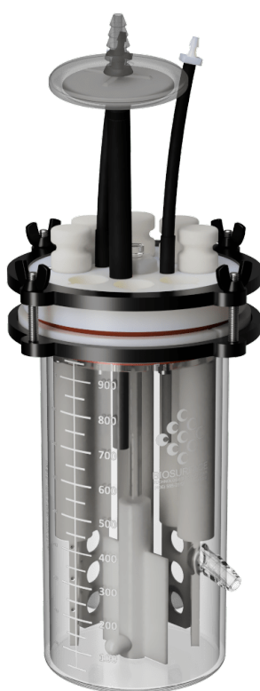
Figure 1.8. CBR 90-3 Anaerobic CDC Biofilm Reactor® (key dimensions: 22 cm reactor height and 12 cm internal diameter; 21 cm coupon holder rod; 1.27 cm coupon diameter) Includes seals around each rod and between lid and vessel. The anaerobic CBR includes coupon holder rods, polycarbonate coupons, coupon removal tool, coupon manipulation tool, and glass flow breaks [181].
