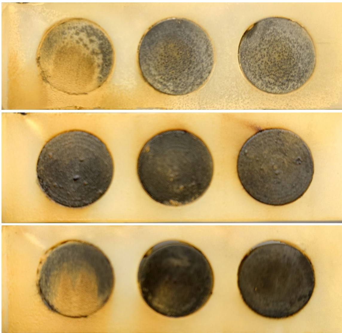
Figure D2a. Photographs taken of the coupon rods taken from the abiotic condition on Day 28, on dismantling the reactor, after exposure to anaerobic produced water media for 28 days.
