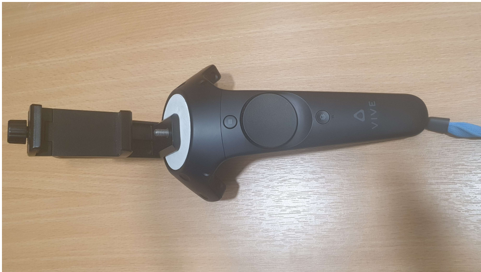
FIGURE 5.5: The controller, the 3D printed holder, and a phone mount
