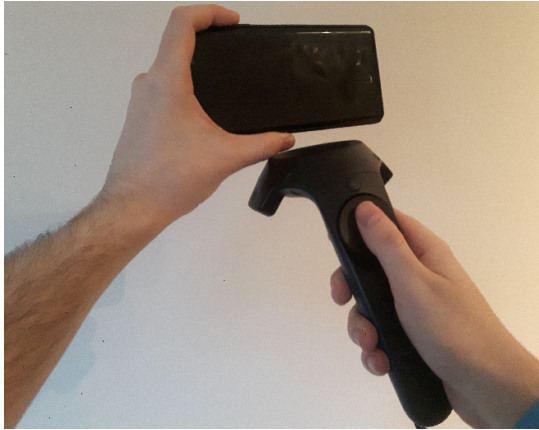
FIGURE 3.4: Phone player uses a phone in one of their hands and a controller to track their position in the other (no need for any holder as we wanted this to be as accessible as possible)
