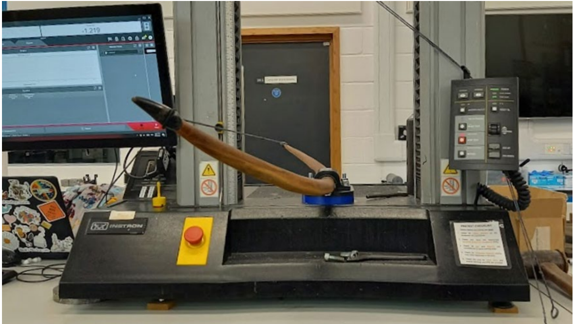
Figure 3-5 Warping of 21MRA5 after submersion in water. In this position the limbs should be curved directly up with the string between them, as in Figure 3.2, so the limbs are warped to the left. Photo: Author.
