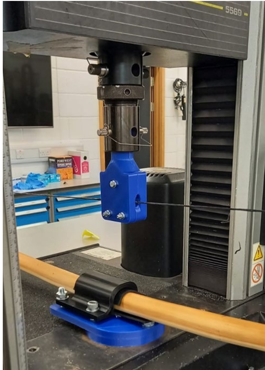
Figure 3-1 Set up for testing the longbows using the custom designed grips to secure the longbow to the base of the machine and the string to the load cell. Photo: Author.
