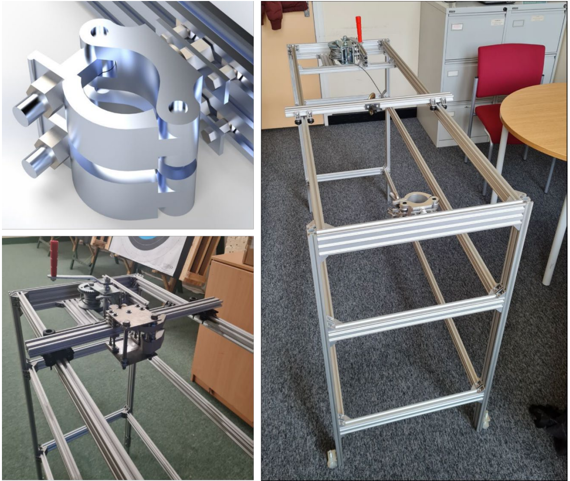
Figure 4-1 a (top left) CAD model of longbow holder subsystem. 4-1b (bottom left) improved trigger design attached to machine. 4-1c (right) complete assembled machine.
