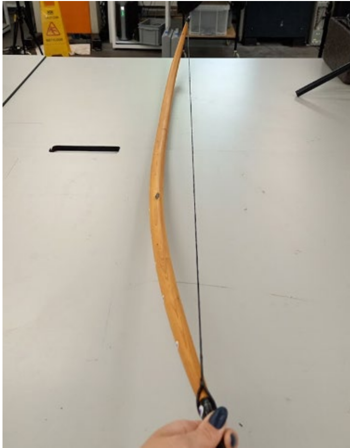
Figure 3-4 Warping of 21MRA1. Held in this position the longbow should be curved underneath the sting, as in Figure 3.2, so the limbs here are twisting to the right. Photo: Author
