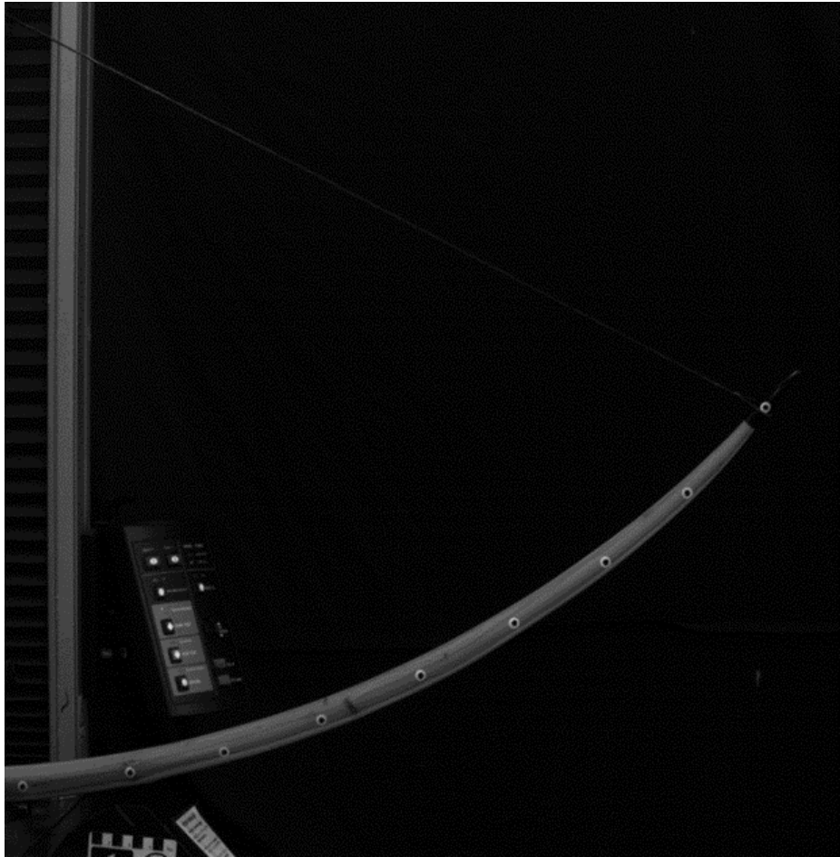
Figure 3-3 Example of the photographs captured by the camera to be used for point tracking. Longbow shown is 21MRA5 at full draw. Photo: Author
