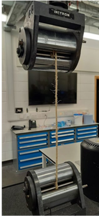
Figure 3-6 Sample of hemp bowstring secured at the top and bottom in cor-de-chasse grips ready for testing. Photo: Author
