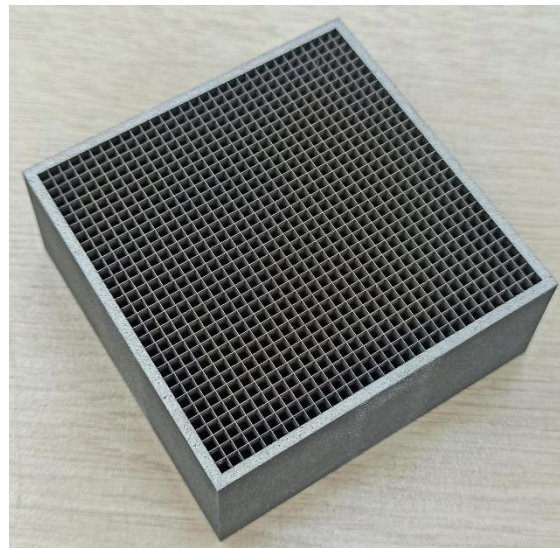
Figure 1: Additively manufactured tungsten 2D focused ASG.
