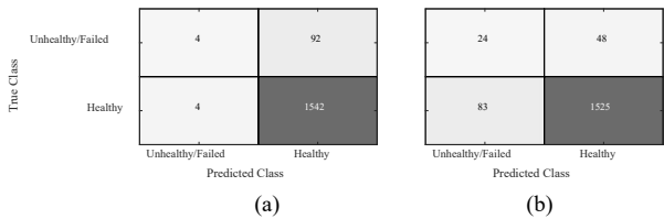
Fig. 11. The classification results obtained via the initial IR guidelines used by the electricity company for (a) 22 kV and (b) 6.6 kV cables.
