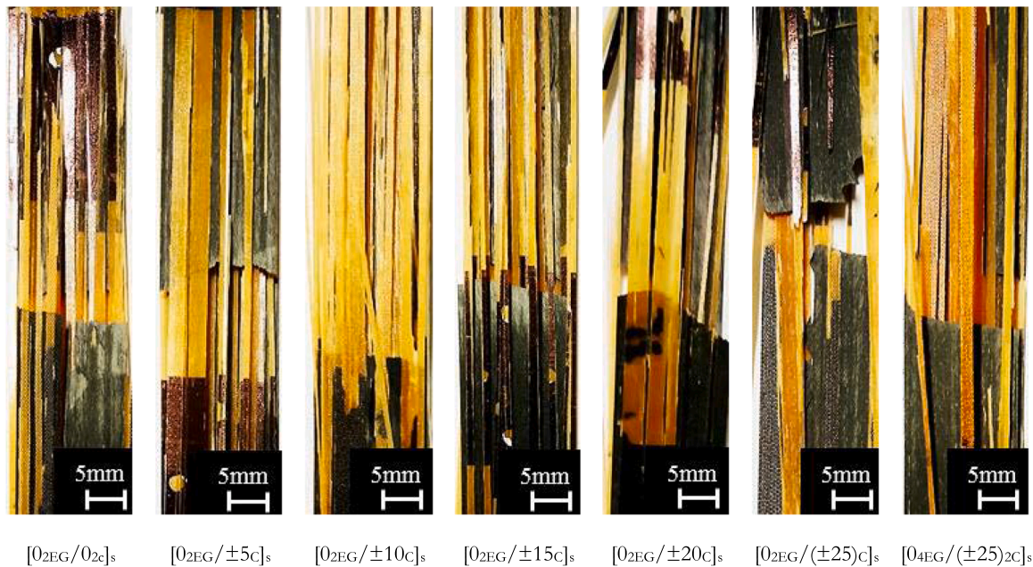
Fig. 8. Samples with different fibre orientations of q = 0^\circ, 5^\circ, 10^\circ, 15^\circ, 20^\circ, 25^\circ (8 plies and 16 plies) after final failure indicating crack in the carbon layer occurring far away from the end-tabs.
