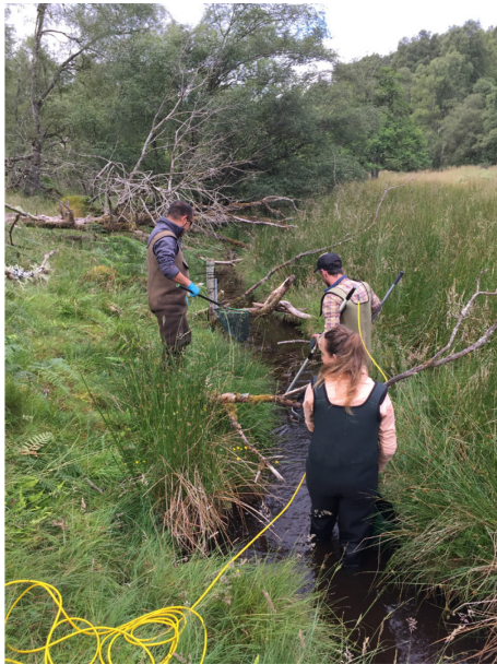
Figure 4.1 Bank based electric fishing using a generator. Note one operator with anode (centre), one operator behind to catch any missed fish and a bank operator to assist with netting of fish and operation of the generator.
