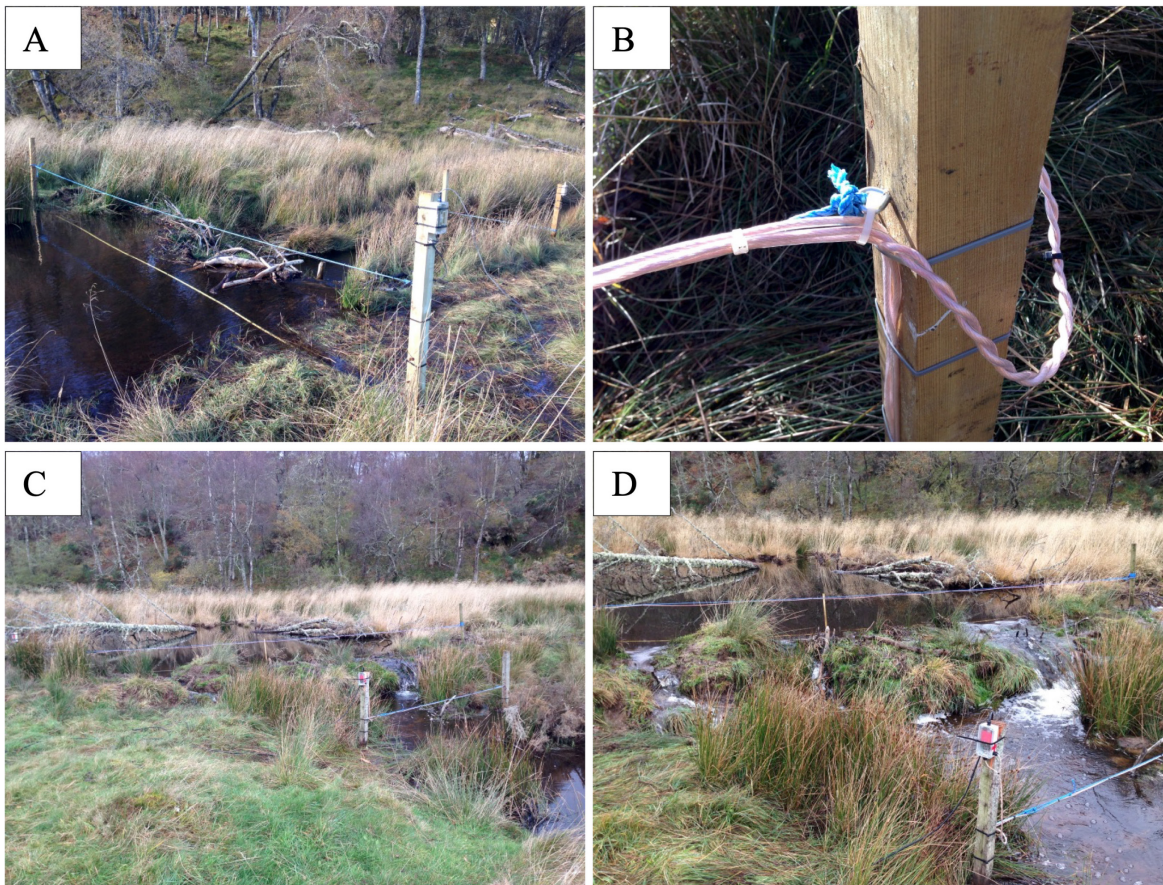
Figure 4.7 [A-D] Passive Integrated Transponder (PIT) telemetry antennae construction. (A) demonstrating the up and downstream PIT antennae at Beaver Dam 1; (B) illustrates how the antennae is framed using nylon rope and fence posts and secured using heavy duty metal eyelets and cable ties; (C) shows the up and downstream PIT antennae at Beaver Dam 2 and (D) illustrates Beaver Dam 2 and the possible fish passage routes to the left and right of the image / dam following rainfall (Photos: R. Needham).
