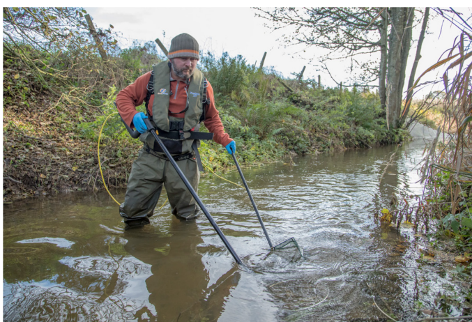
Figure 4.2 Electric fishing using backpack method. Note one operator controls the anode, cathode and net. Note, additional operator out of shot at time of photo.
