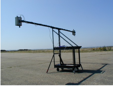
Fig. 2. Mobile spectroradiometer mounting for ensuring positional accuracy in spectral measurements.
