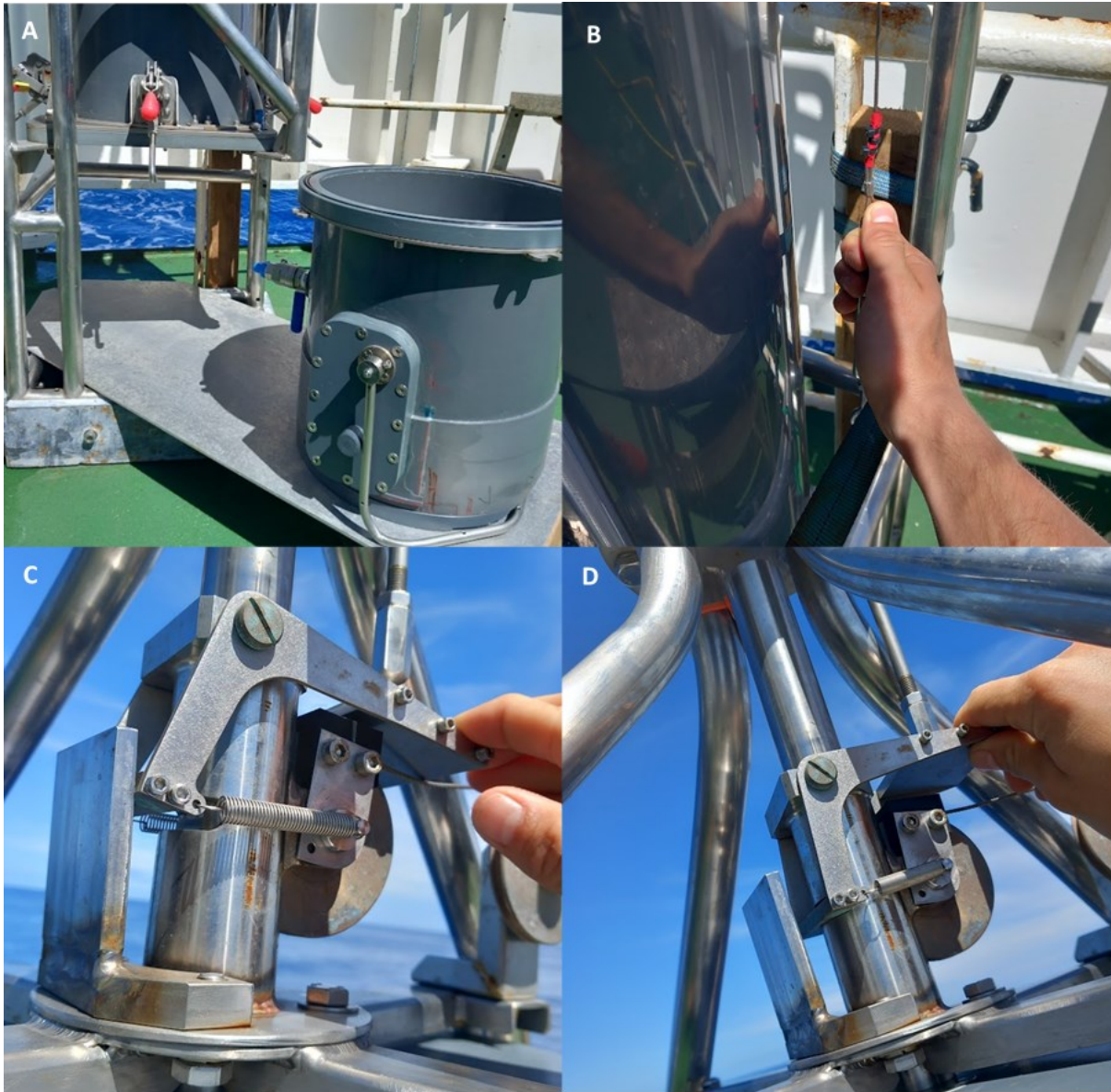
Figure 5.4 Key steps during preparation of MSC Yuki for deployment (a) Inserting the base section of Yuki beneath the upper section using the sliding tray; (b) Pulling down on the metal wire to raise the lid of Yuki; (c) The lid held (by hand) in the raised position, with the pivot plate not inserted into the central pole slot. If released in this position, the lid would fall; (d) lid secured in the upper position with the pivot plate inserted into the groove of the central pole. Holding the pivot in position as shown may also be used when attaching shackle to MSC if not using a wooden wedge, to ensure MSC is not fired accidentally.
