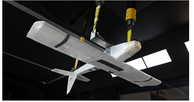
Fig. 1: UAV mounted to wind tunnel overhead balance.
