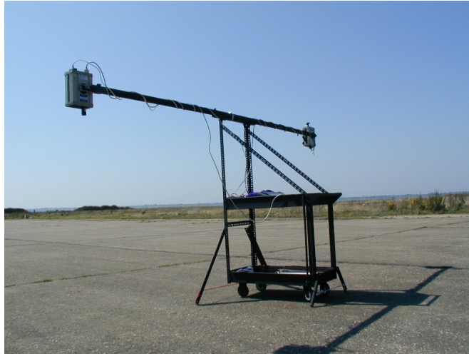
FIGURE 2: Mobile spectroradiometer device for ensuring positional precision in spectral measurements.
