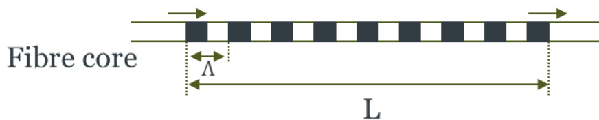
Figure 3.1: Schematic diagram of a SMF-LPFG.
