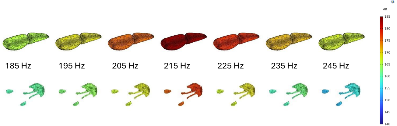
Figure 4.43 Simulated SPLrms of the swim bladder (top) and the otoliths (bottom) at the test frequency of 185, 195, 205, 215 (resonance frequency), 225, 235, and 245 Hz.
