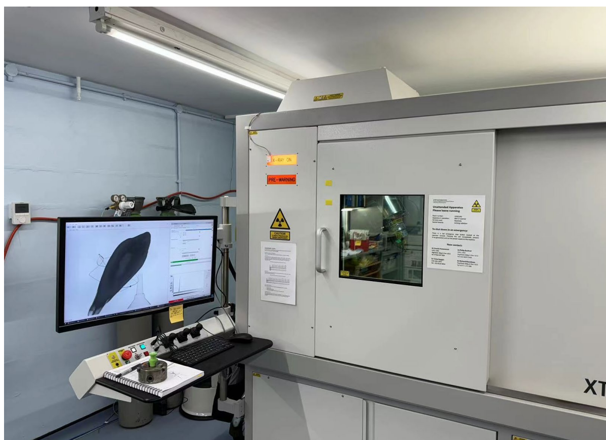
Figure 4.32 Photo of specimen A inside the scanner during the scanning with the monitor showing the real-time raw output image.
