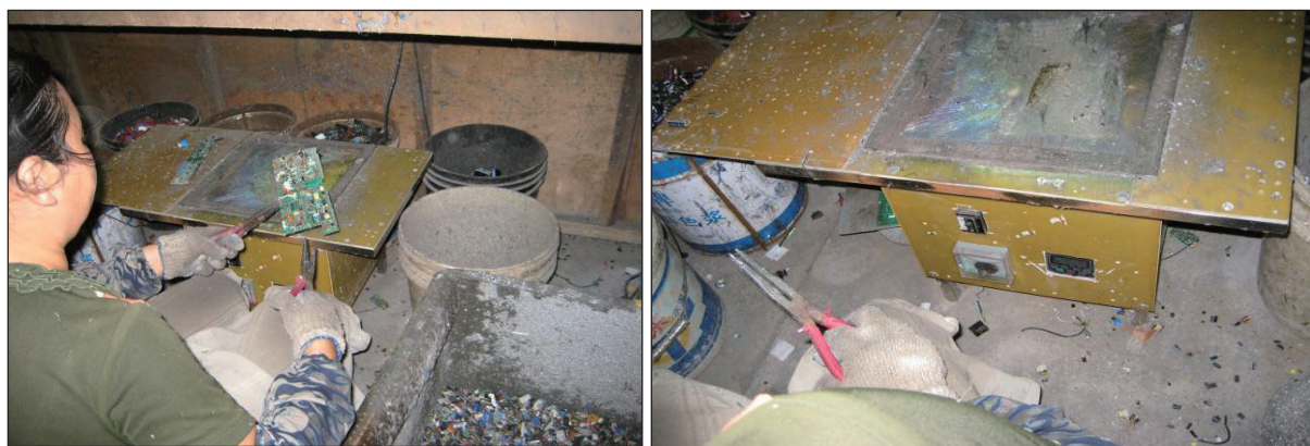
Figure F- 3 Heat the boards over a coal stove with an iron plate or a flat pan (Source: By (Shantou Chaoyang District People's Government, 2010))
