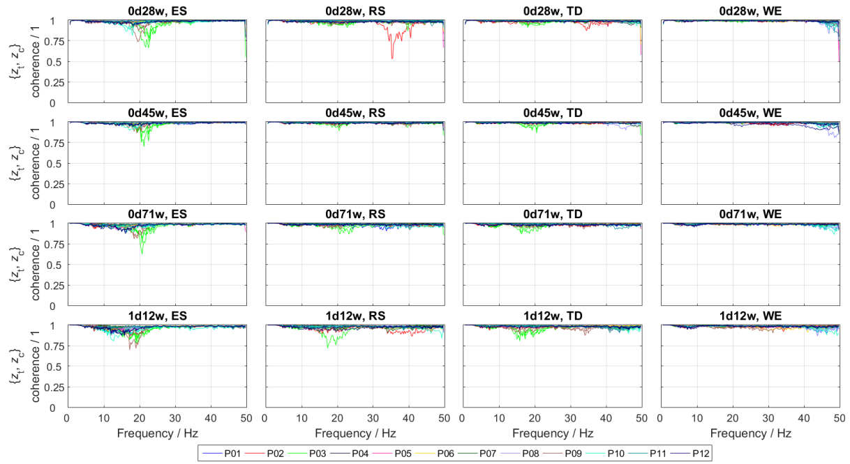
Figure 20 Coherence plots of the response functions ( \{z_t, z_c\} transmissibility and \{z_t, z_c\} coherence) for all 36 tests per treatment. Cells: \{z_t, z_c\} coherence vs frequency. Total sample: 12 participants (six males and six females). Vibration magnitude levels: {0d28w, 0d45w, 0d71w, 1d12w}. Sitting configuration levels: {ES, RS, TD, WE}. Participants: {P01, ..., P12}.
