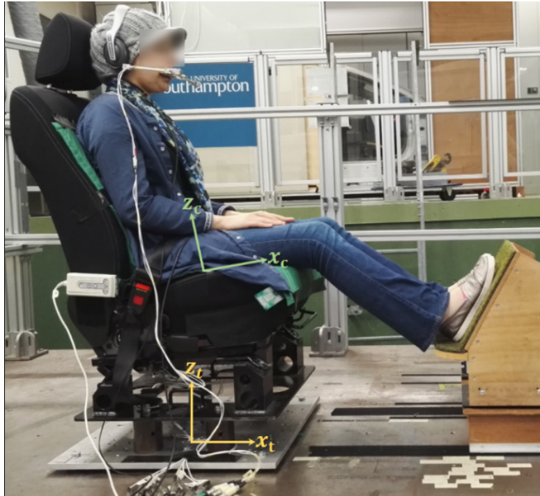
Figure 16 Experimental arrangement and coordinate systems. \{x_t, y_t, z_t\} = coordinate system at vibration table; \{x_c, y_c, z_c\} = coordinate system at interface between seat cushion and occupant buttocks.
