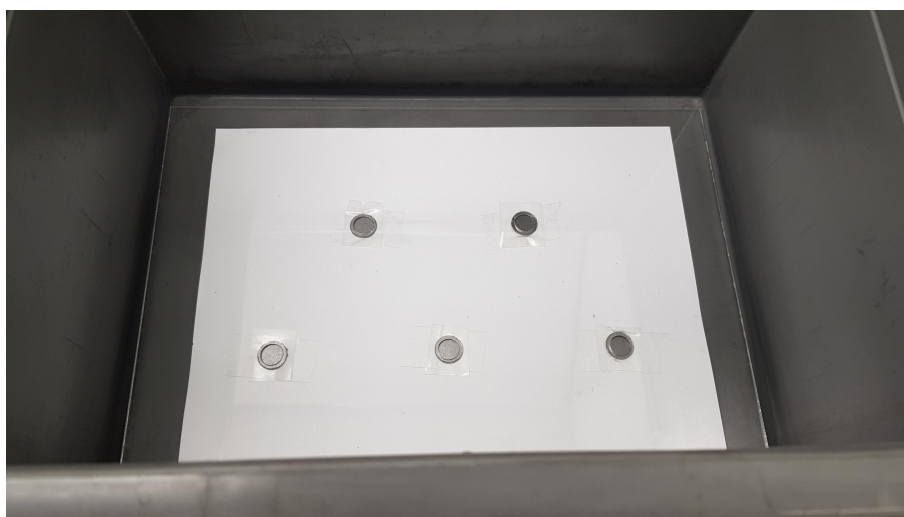
FIGURE 3.9: Spraying mask with electrodes set up pre spraying
