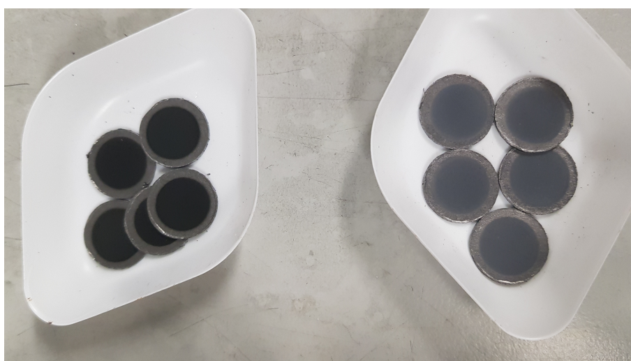
FIGURE 3.11: Final electrodes after removal from mask - left CuHCF electrodes, and right, \text{TiO}_2
