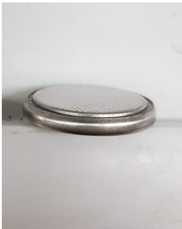
FIGURE 3.16: Final crimped cell
