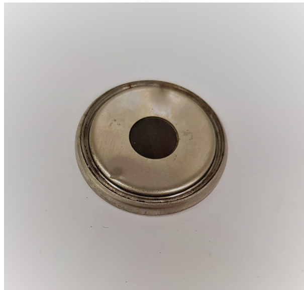
FIGURE 7.3: Crimped cell with laser thinned window on case
