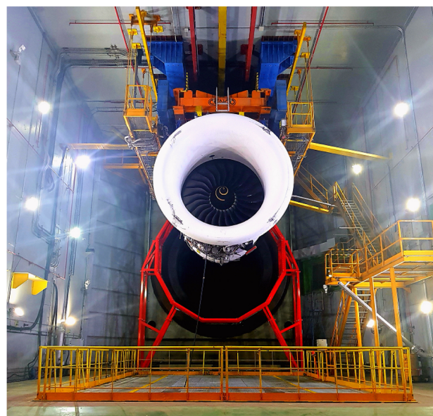
Fig. 1. Optical mounting frame (red) behind a large scale commercial aero-engine at the engine test bed facility at Instituto Nacional de Técnica Aeroespacial (INTA), Madrid.
