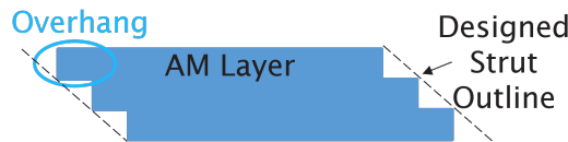
FIGURE 3.8: Stair-stepping diagram for angled struts
