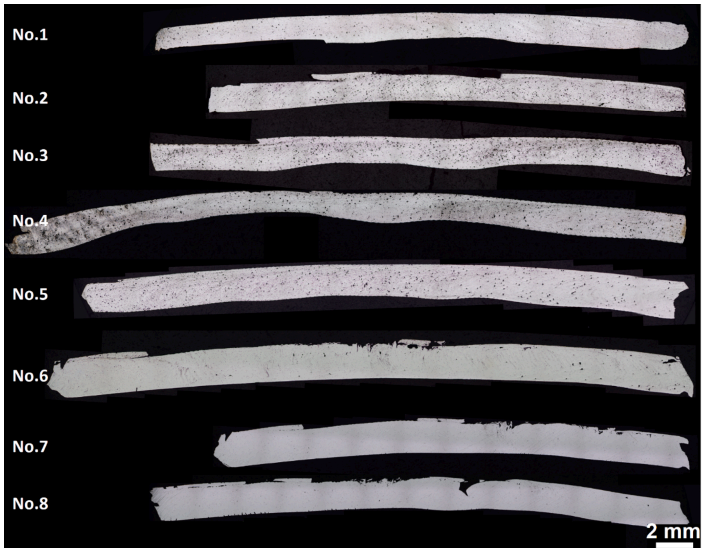
Fig. 5. Stitched OM images of all the 8 cross-sections in the extruded wire, with Section No.1 at the top to Section No.8 at the bottom.
