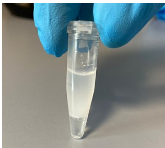
Figure S3: photo of a nanodroplet solution consisting of 20 %vol PFP after the second sonication at a tip height of 2mm. The separate phases of the PFP at the bottom and the lipid film above can be seen clearly
