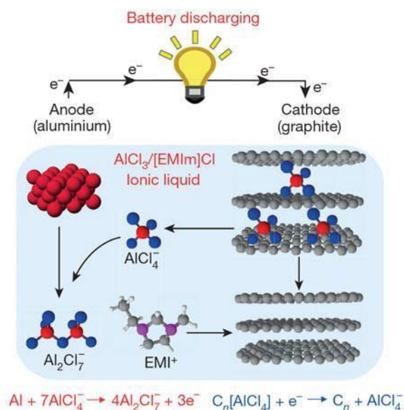
Figure 2.11 Operation mechanism of the Al-graphite battery. During discharge, \text{AlCl}_4^- anions deintercalate from the graphite host at the cathode, while at the same time \text{AlCl}_4^- react with Al at the anode yielding \text{Al}_2\text{Cl}_7^- (Al dissolution). The reverse process occurs upon charging, where Al is electrodeposited at the anode and \text{AlCl}_4^- anions undergo intercalation into the graphite cathode. Reproduced with permission from [41]. Copyright 2015, Springer Nature Limited.
