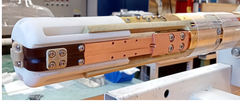
FIGURE 3.7: U-shape sample holder mounted on the solenoid insert. The white piece is used to add rigidity to the holder, but later revealed to be unnecessary.
