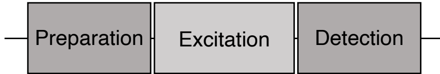
FIGURE 1.3: The basic anatomy of an NMR experiment.
