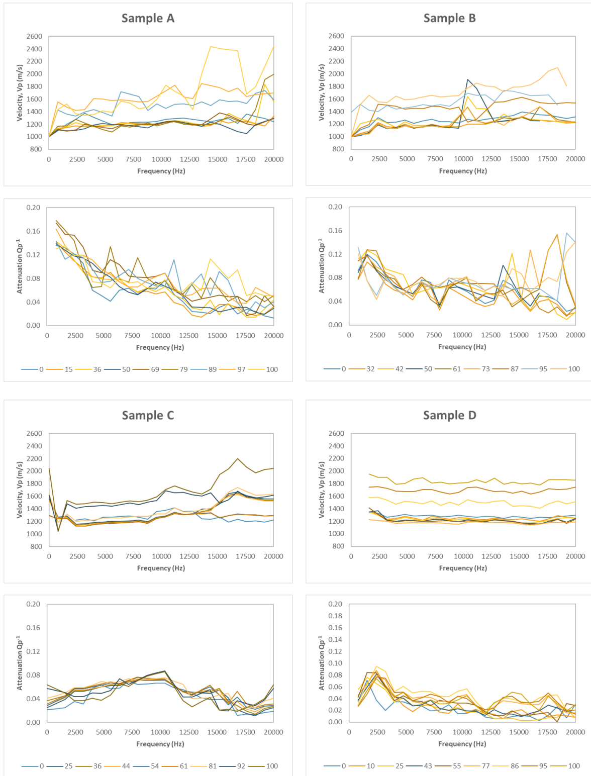
Figure D.5 Variations in P-wave velocity ( V_p ) and attenuation Q_p^{-1} across a frequency range of 1-20 kHz, with legends at each plot represent the saturation levels. The measurements were conducted under an effective pressure of 10 MPa and a temperature of 4°C.
