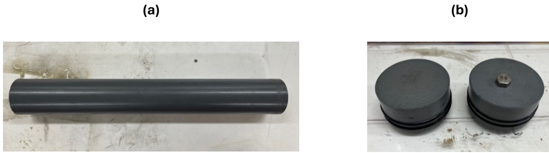
Figure F.1 PVC jacket system used to enable sample emplacement inside the water-filled acoustic pulse tube: a) 50 cm length PVC cylinder jacket, and b) top and bottom PVC endcaps with O-ring seals, including the location of the pore fluid vent port (shown as a hexagonal nut on the top endcap on the right).
