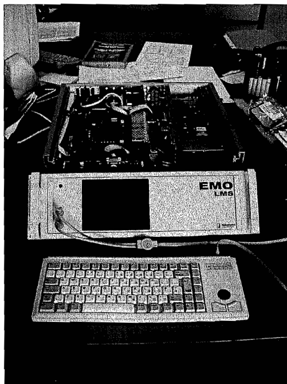
Figure 2.3.5 Improved detection system and signal processing unit, (Built by industrial sponsors). Shown above is a picture of the improved EMO detection unit, built by the industrial sponsors of the work presented in this thesis. This unit incorporates a DDC unit. The output is then sampled by a PC also included in the unit. The data is then processed and displayed simultaneously on the screen on the front of the unit. A frequency reference is recovered from a GPS signal. This unit also has satellite phone capabilities to communicate with the mobile magnetic field generator.
