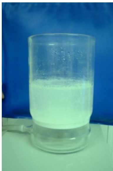
Figure 3.21 The fast response gas bubbler in operation. A beaker is divided by a large-area glass sinter. The lower chamber is pressurised with an air/nitrogen mixture which bubbles into the water sample above. The bubbler was photographed while an air/nitrogen mixture was bubbled through the test water sample.
