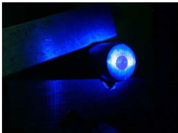
Figure 6.1 Oxygen probe illuminated with 470nm blue LED light after 16 hour test. The sensing membrane is the smaller disc glued to the end of the probe
