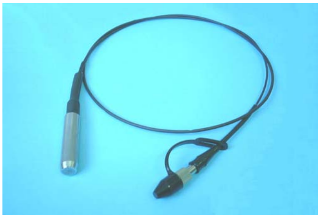
Figure 2.5 Probe (left), 2m connecting fibre lead, and modified (for low auto-fluorescence) 'FC' type fibre connector (right). The probe body measured 70x8mm.
