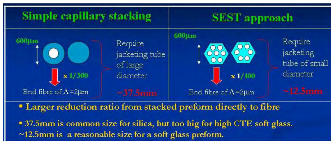
Figure 5.8: Comparison of CAST and SEST HF's on the fibre drawing reduction ratio
