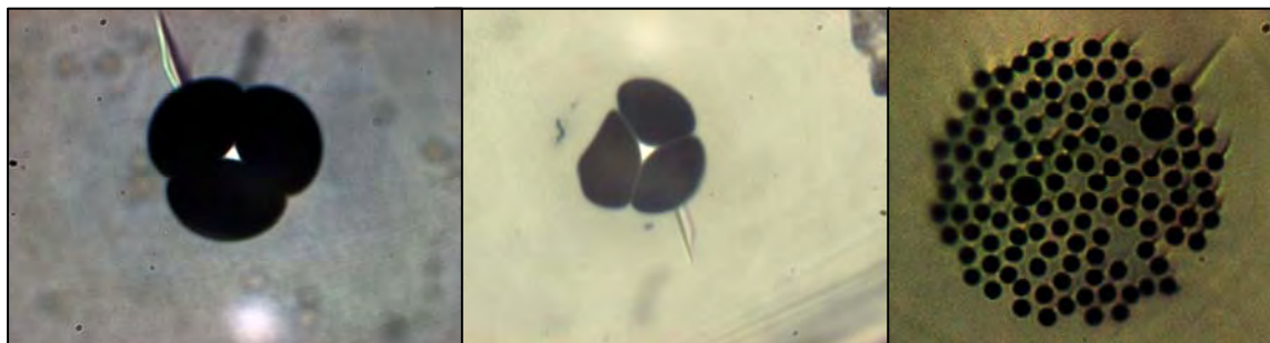
Figure 3.2: Optical microscope images of some badly cleaved fibres. Note the imperfections around the holes and the cracks running between some of them.
