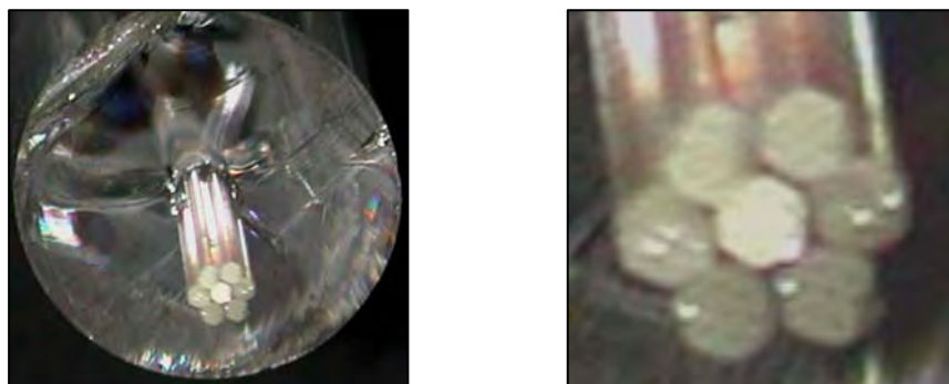
Figure 5.16: The stack is tightly fitted inside the jacketing tube.
