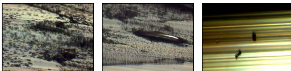
Figure 3.8: Optical microscope images of impurities (black particles) found in some extruded fibre preforms (these fine particles are in micron scale).
