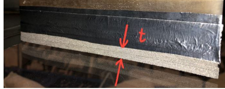
Figure 2.2: Photo of a porous tip treatment of thickness t across the entire chord.
