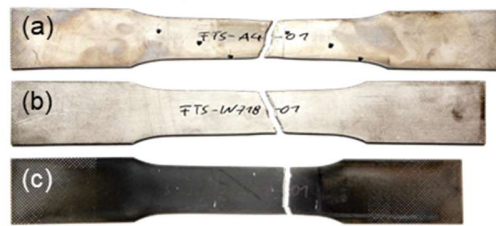
Figure 8. Specimen tensile test: (a) stainless steel (1.4571); (b) Inconel 718 (Plate); (c) Inconel 718 (SLM).
