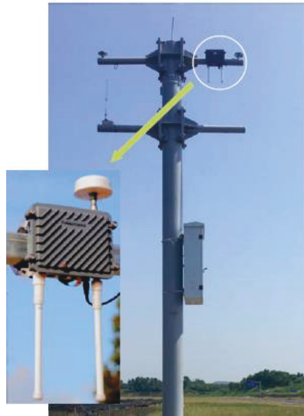
Figure 2-3 Roadside Unit. From Chen et al. (2018).
