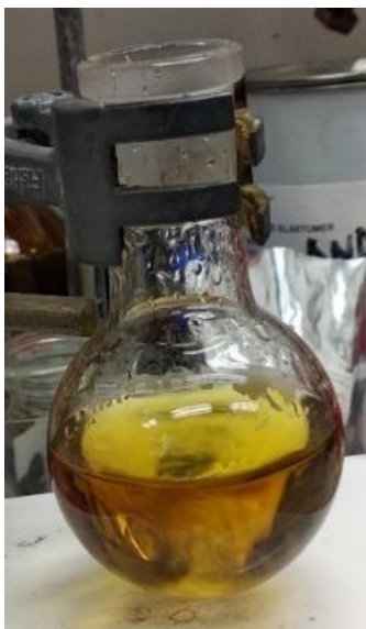
Figure 3.2. Colloidal solution of Ag seeds
