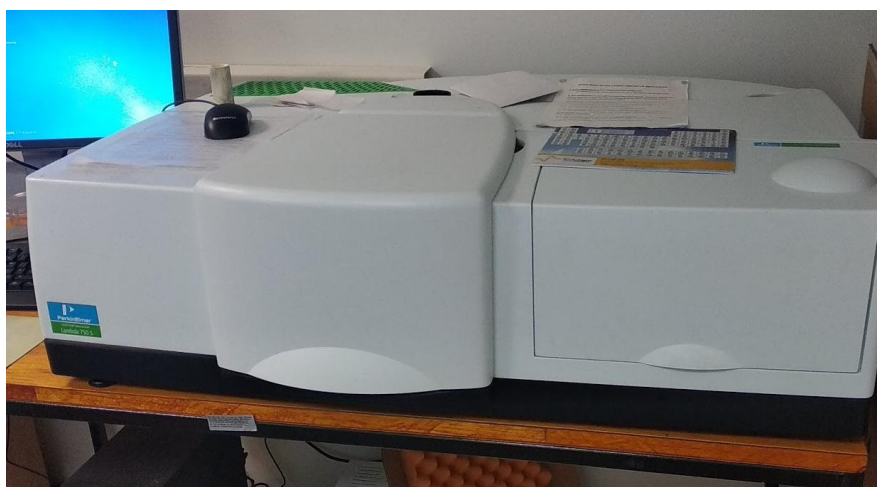
Figure 3.6. Perkin Elmer Lambda 750S UV-VIS-IR spectrophotometer
