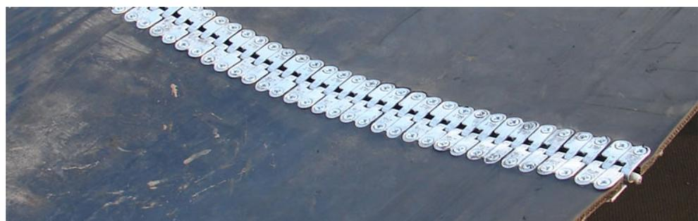
**Figure 7.** Belt joint using a metal clip.
