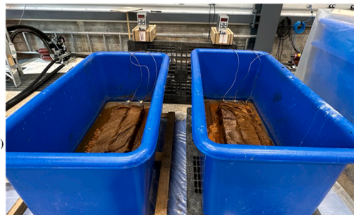
Fig. 7. The accelerated corrosion process conducted in this study.
