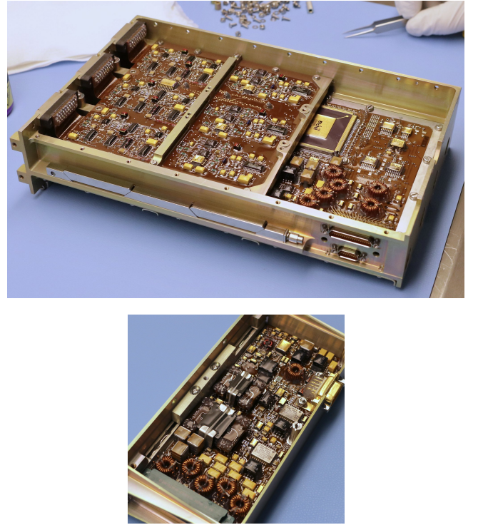
Fig. 13. VIS Readout Electronics ( top ) and Power Supply Unit ( bottom ). The Readout Electronics consists of two double-sided circuit boards containing the 12 analogue channels – three repeating analogue circuits can be seen in the topmost board – with the digital board containing the Field Programmable Gate Array between them and to the rear of the unit. The connectors to the upper flexible connections from the CCDs are at the front of the unit. The Power Supply Unit contains also a tightly populated double-sided circuit board. The planar transformers can be seen on the centre-left of the unit.
