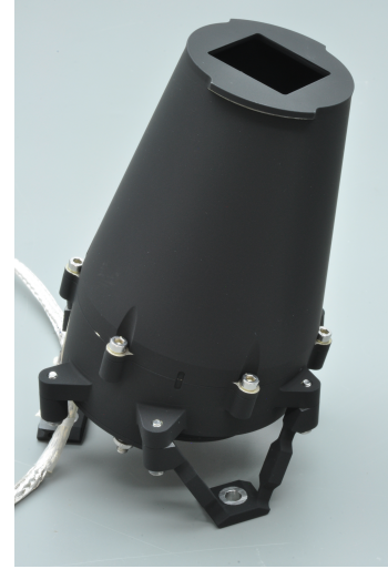
Fig. 13. Flight model of the calibration source NI-CU before integration into NISP. Two supply harnesses can be seen, feeding the nominal and redundant side, respectively, of NI-CU with each five LEDs emitting at different wavelengths. Inside the base any LED illuminates the same PTFE reflector patch that in turn directly illuminates the FPA, with a field shaped by a set of five baffles, the last one visible at the top. The full NI-CU height is approximately 150 mm.
