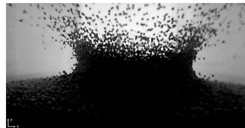
Fig. 12. Side view of a 100 ms pulse steel bead experiment in microgravity by Chambers et al. in 2020 [26].
