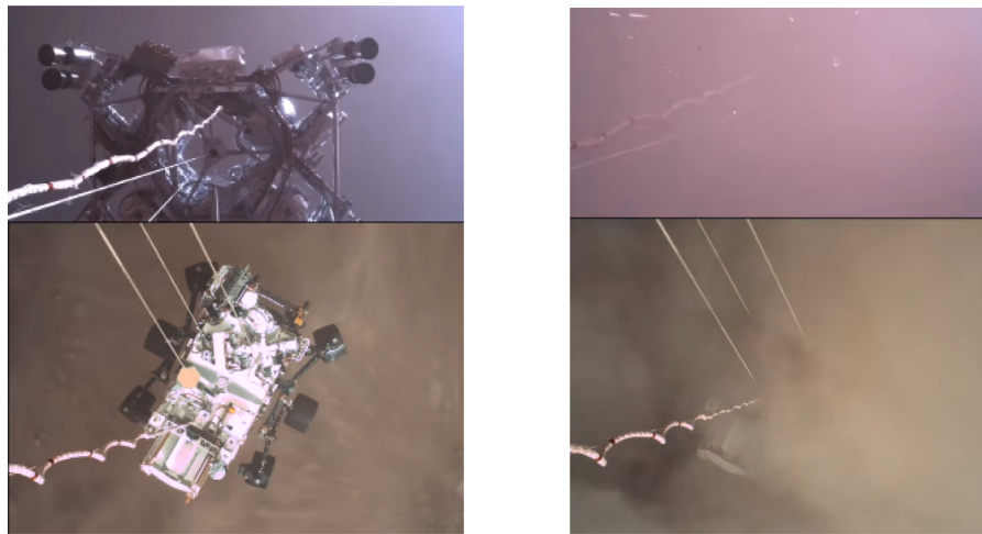
(a) Descent stage (top) hovers using retro-rockets and lowers the rover (bottom). (b) Onboard cameras are obstructed by lofted surface particles.
