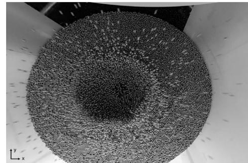
Fig. 11. Top-down view of a 50 ms pulse steel bead experiment in microgravity by Chambers et al. in 2020 [26].
