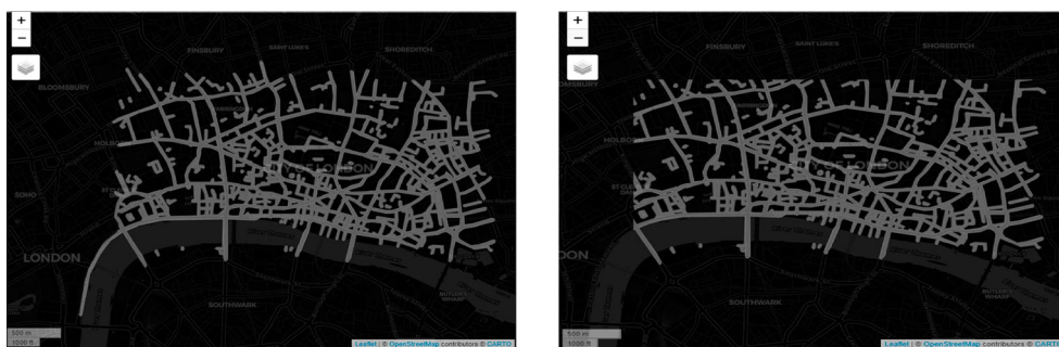
Figure 5. (Left) OSM road network with a 20 m buffer; (Right) Clipped polygon of buffered segments.
