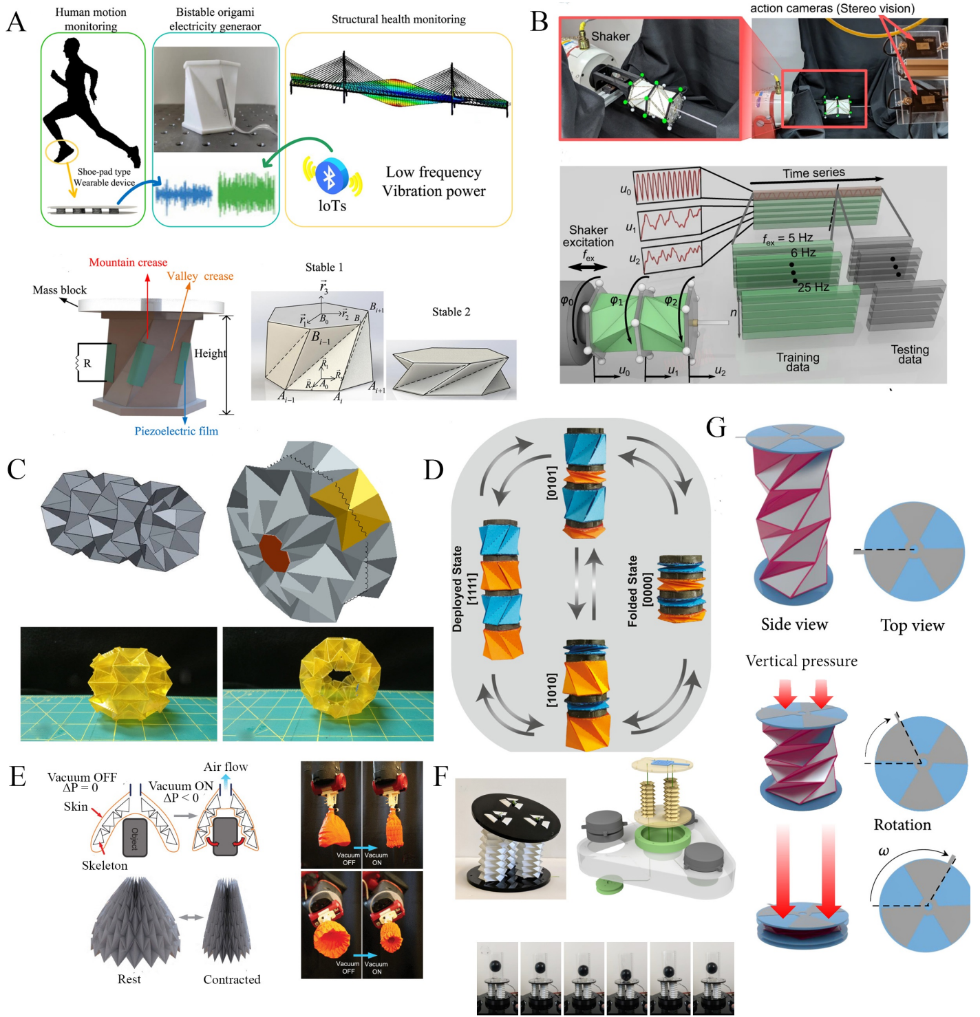
Figure 4: Multiple functionalities of tubular origami metamaterials. (A) Bistable Kresling origami energy generator for wearable devices and bridge monitoring devices [154] (B) Two triangulated cylindrical origami used in a vibrating environment to analyze and control the dynamic behaviour [155] (C) Waterbomb origami wheel with shape memory alloy actuator for variable functionalities [143] (D) Untethered origami microrobots with magnetic actuation [156] (E) Waterbomb origami inspired magic ball soft gripper with pneumatic actuator [144] (F) A three limb juggler based on reconfigurable expanding bistable origami [138] (G) A piezoelectric/triboelectric energy generator based on triangulated origami cylinders [157].
