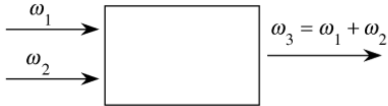
FIGURE 1.1: Geometry of frequency upconversion, a phenomena whereby a nonlinear material can convert input light with frequencies \omega_1 and \omega_2 to a different frequency \omega_3 , defined by \omega_1 + \omega_2 = \omega_3 .
