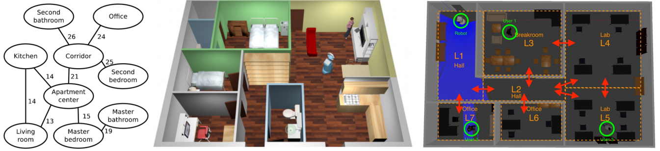
Fig. 2: Left: Topological map of Aruba environment [16]. Center: Simulation of Aruba environment by [16]. Right: Realistic office environment simulated in Gazebo including TIAGo and three users. Significant locations are marked, the blue shaded area shows the robot's rangefinder's visibility.
